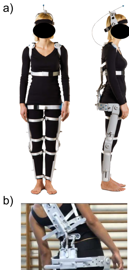
Figure 1. The Human Body Posturizer (HBP) orthosis. a) Frontal and lateral view of the HBP exoskeleton worn by an actor. b) Close-up of the rear view showing the articulation capacities. The subject of the photograph has given written informed consent, as outlined in the PLOS consent form, to publication of their photograph. doi:10.1371/journal.pone.0077348.g001
