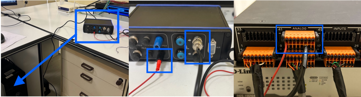
Figure 5.3. Hardware setup used for stimulus triggering and synchronization during the unplanned Functional Reach (unplFR) task. The Trigger Box was connected to the laboratory computer via USB and to the Vicon Lock system via analog inputs.
