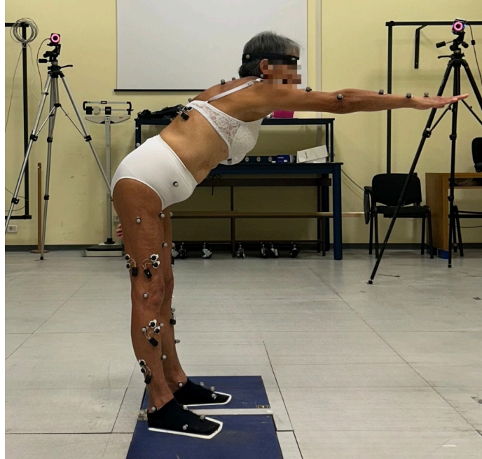
Figure 10.1. Experimental set-up for the Functional Reach task. The figure shows a representative older adult participant instrumented with surface electromyography (EMG) electrodes and infrared reflective markers. EMG electrodes were placed bilaterally over eight muscles: anterior deltoid (AD), erector spinae (ES), latissimus dorsi (LD), vastus lateralis (VL), tibialis anterior (TA), biceps femoris (BF), gastrocnemius medialis (GastM), and soleus (Sol). A total of 61 infrared reflective markers were positioned according to the Plug-in Gait and Conventional Gait Model 2.5 kinematic protocols. Whole-body kinematics were recorded using an optoelectronic motion capture system.
